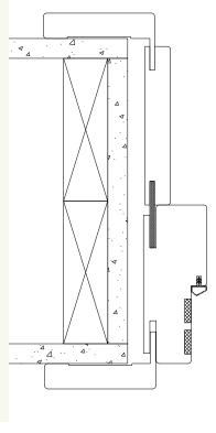
Instances where the wall is of greater depth than the frame (typically a corridor) where such that the architraves are trimmed to abut the wall reveal face.
