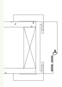
Instances where the wall thickness is greater than the frame and an extension lining is not preferred. The frame is flush to one face of the wall such that the pull side architraves are fitted flat to the wall face and the push side architraves are trimmed to abut the wall reveal face.
