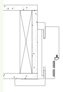
Instances where the wall thickness is greater than the frame (between 70mm and 110mm) and an extension lining is used. The frame is flush to one face of the wall such that the architraves are fitted flat to both faces.
