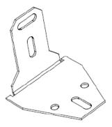
The brackets shall be fitted at a maximum of 120 mm from the top and bottom corner of each jamb, and at maximum 450 mm centres.
