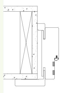
Instances where the wall thickness is greater than the frame (between 70mm and 110mm) and an extension lining is used. The frame is flush to one face of the wall such that the architraves are fitted flat to both faces.
