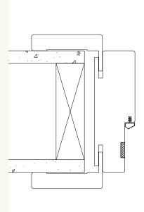
Instances where the wall thickness is greater than the frame and an extension lining is not preferred. The frame is flush to one face of the wall such that the pull side architraves are fitted flat to the wall face and the push side architraves are trimmed to abut the wall reveal face.
